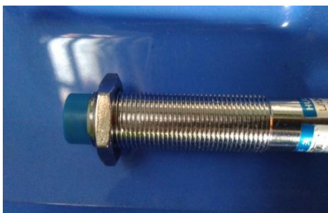
Gambar 7. Sensor Proximity Inductive
