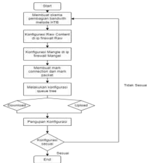
Gambar 3 Flowchart Alur Perancangan HTB
