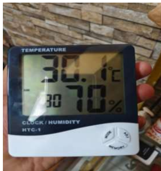
Gambar 4. Alat ukur suhu dan kelembaban seri HTC-1 KF90 UVI and Radiation Meter
